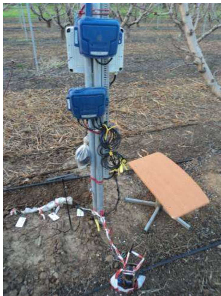
The images above report the installation of soil moisture probes.
