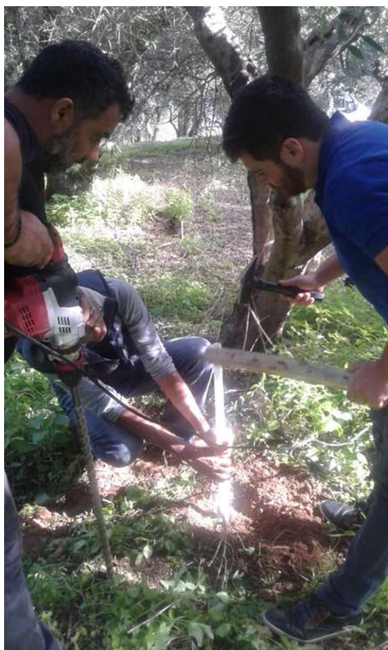
Figure 23. Access tubes installation for soil moisture measurements
