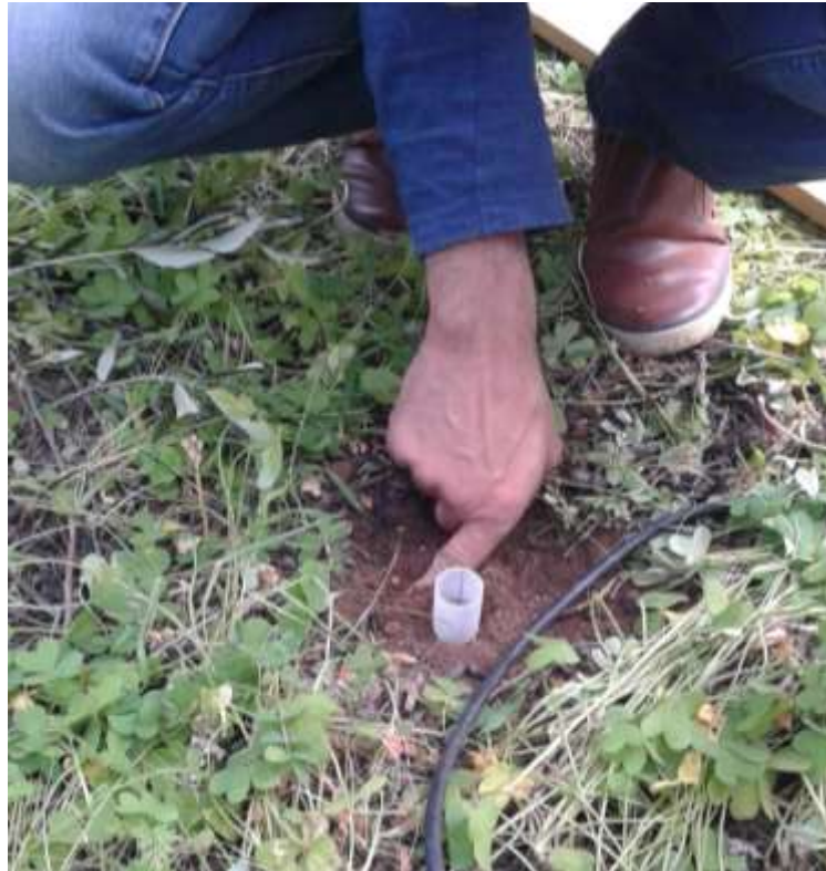
Figure 4. Access tubes installation for soil moisture measurements
