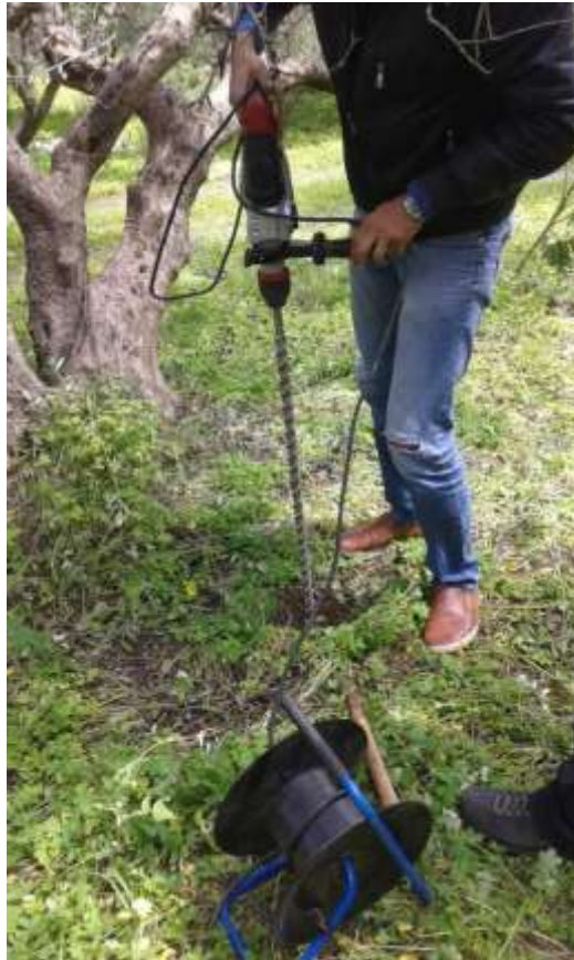
Figure 15. Access tubes installation for soil moisture measurements
